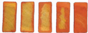
Under ideal conditions, Bora-Care penetrates wood over a 4-6 week period and remains for the life of the wood.
